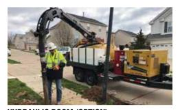
**HYDRAULIC BOOM (OPTION)** The hydraulic boom offers a 6-way function, wireless remote with vacuum valve operation, 330-degree rotation, remote water jet for easy cleanout, and a 5" hose with quick connect to 4" tooling.
