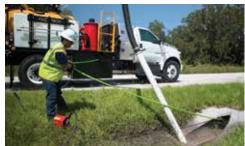
**JETTER PACKAGE** 15 gpm @ 3,000 psi water pump with 425' x 1/2" jetter hose that comes with electric self-retracting hose reel.
