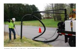
**STRONG ARM (OPTION)** With 270-degree rotation, the strong arm supports the weight of the vacuum hose and the roller head makes handling much easier by allowing smooth, fluid movements and adjustments.
